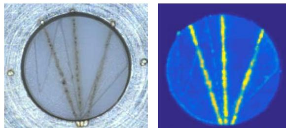
**Figure 1.** RLS CT with pattern (left). Characterization of the RLS CT with the RLS ExoMars Simulator (right)
