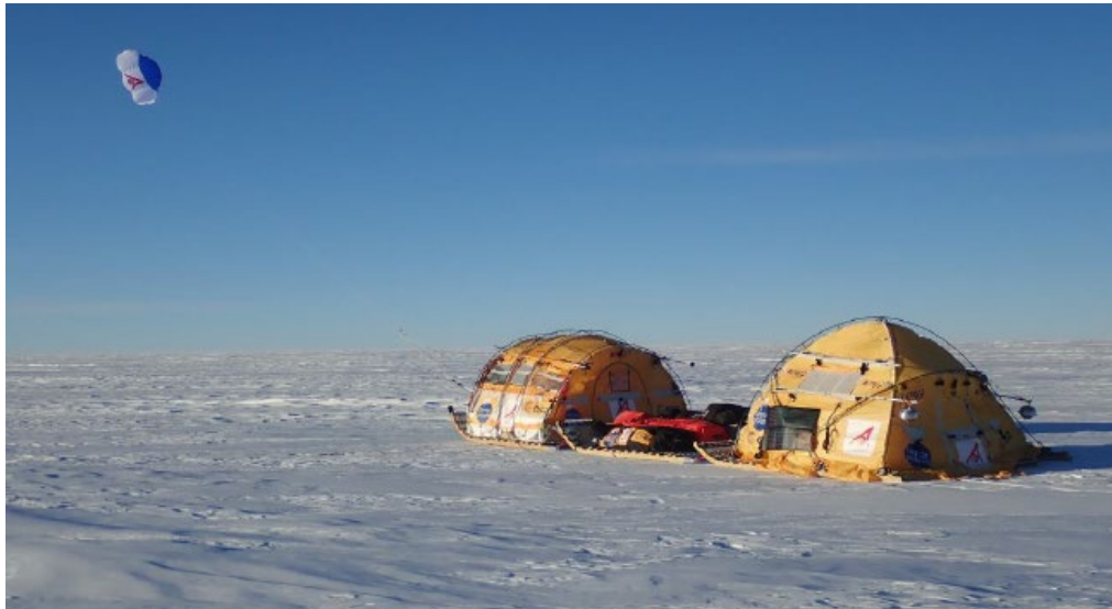
WindSled propelled by wind on the Antarctic Plateau
