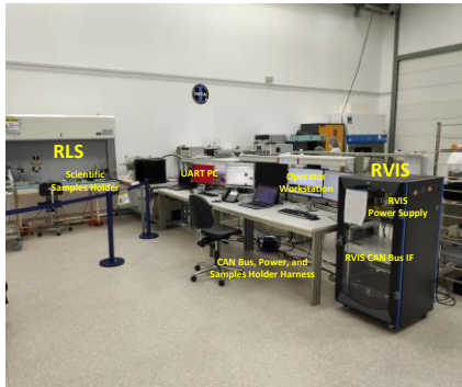
Figure 2. Testing framework inside INTA facilities
